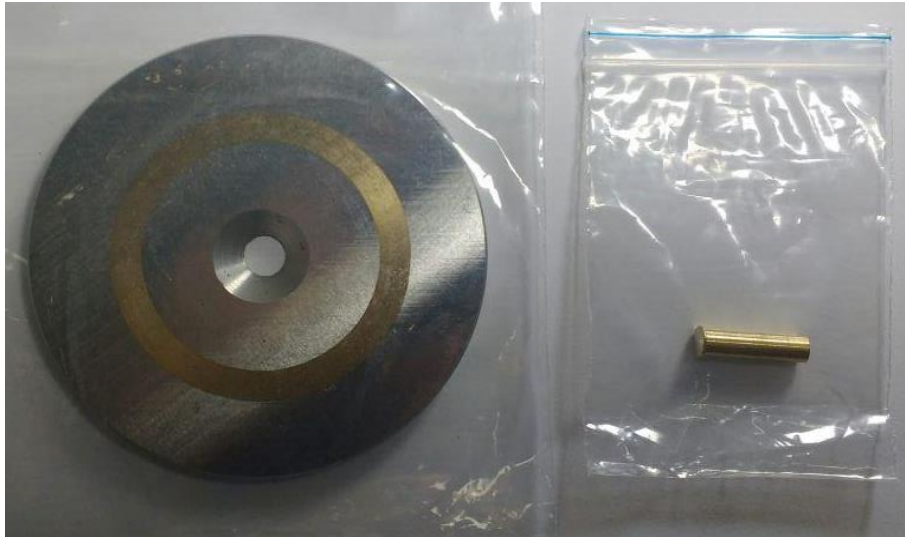
Figure 8: Brass pin and steel disc tested under 2.55 MPa (50N normal load).
