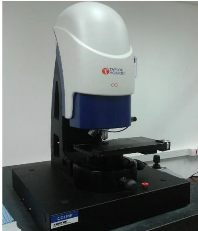
Figure 9: Taylor Robson CCI 3D-profilometer.
